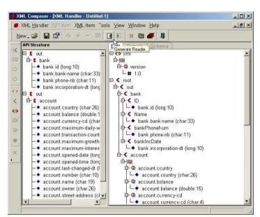
XML Composer's visual designer allows the mapping of EAB information views to XML elements and attributes. The XML data structure can also be manipulated easily in a visual design environment, allowing developers to design XML data handling programs without having to perform low level programming. Source code is automatically generated to implement the mappings between attributes in the EAB Views and the desired XML elements/attributes.
